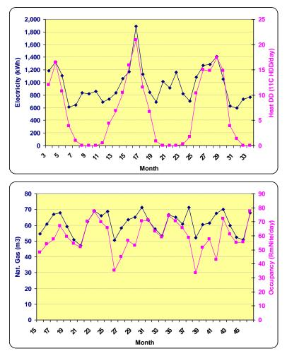
represent the full relationships for each of gas and electricity. These equations could be used to budget energy consumption on the basis of weather or occupancy and to monitor future consumption to detect future savings.
